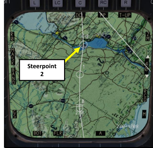
TSD (Tactical Situation Display) Page Steerpoint "2" (Not converted to Target Point)
