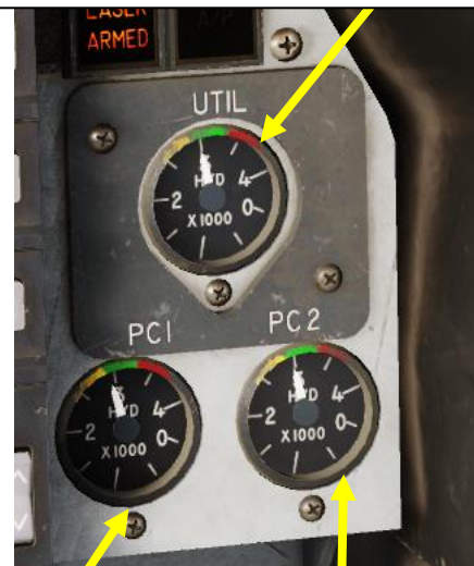
PC1 (Power Control 1) Hydraulic System Pressure Indicator (x1000 psi)
