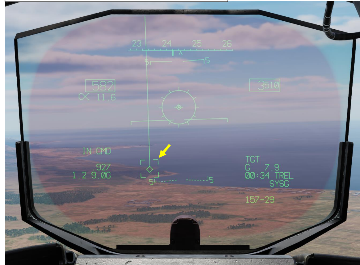
Targeting Pod Slaved to HUD Designation from Auto Mode TD (Target Designation) Box
