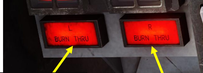
Left Engine Afterburner BURN THRU Warning Light • Illuminates when burn through or overtemperature condition in the left engine's afterburner section is detected
