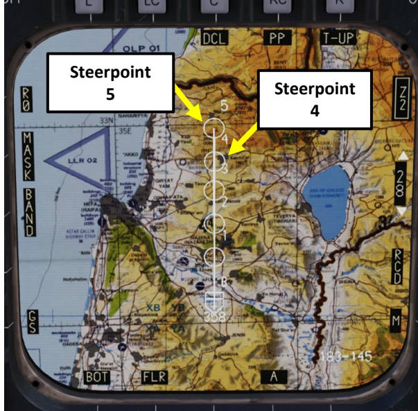
TSD (Tactical Situation Display) Page Steerpoint “5” (Not converted to Target Point)
