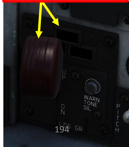
Landing Gear UP & LOCKED
