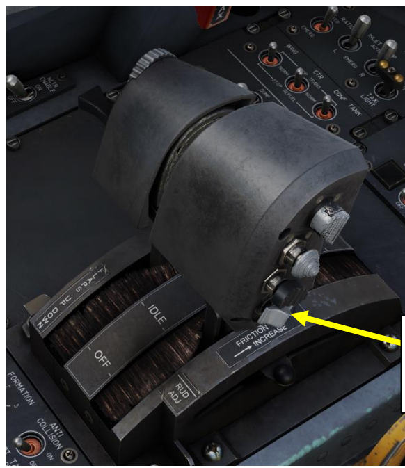
Weapon / Mode (Weapon Select) Switch • FWD: Medium Range Missile Selected • CENTER: Short Range Missile Selected • AFT: Auto Guns / A/A Mode Command Selected
