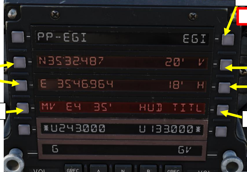
2b PPKS (Present Position Keeping Source) Sub-Menu
