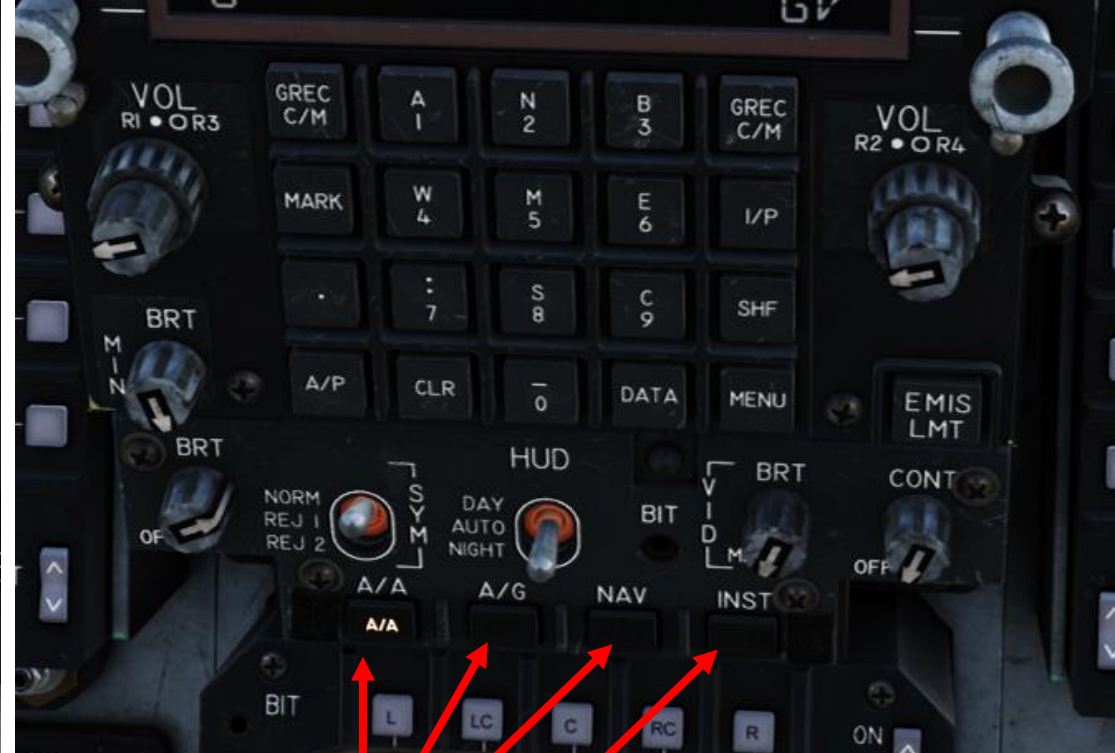
Master Mode Buttons • A/A: Air-to-Air • A/G: Air-to-Ground • NAV: Navigation • INST: Instrument
