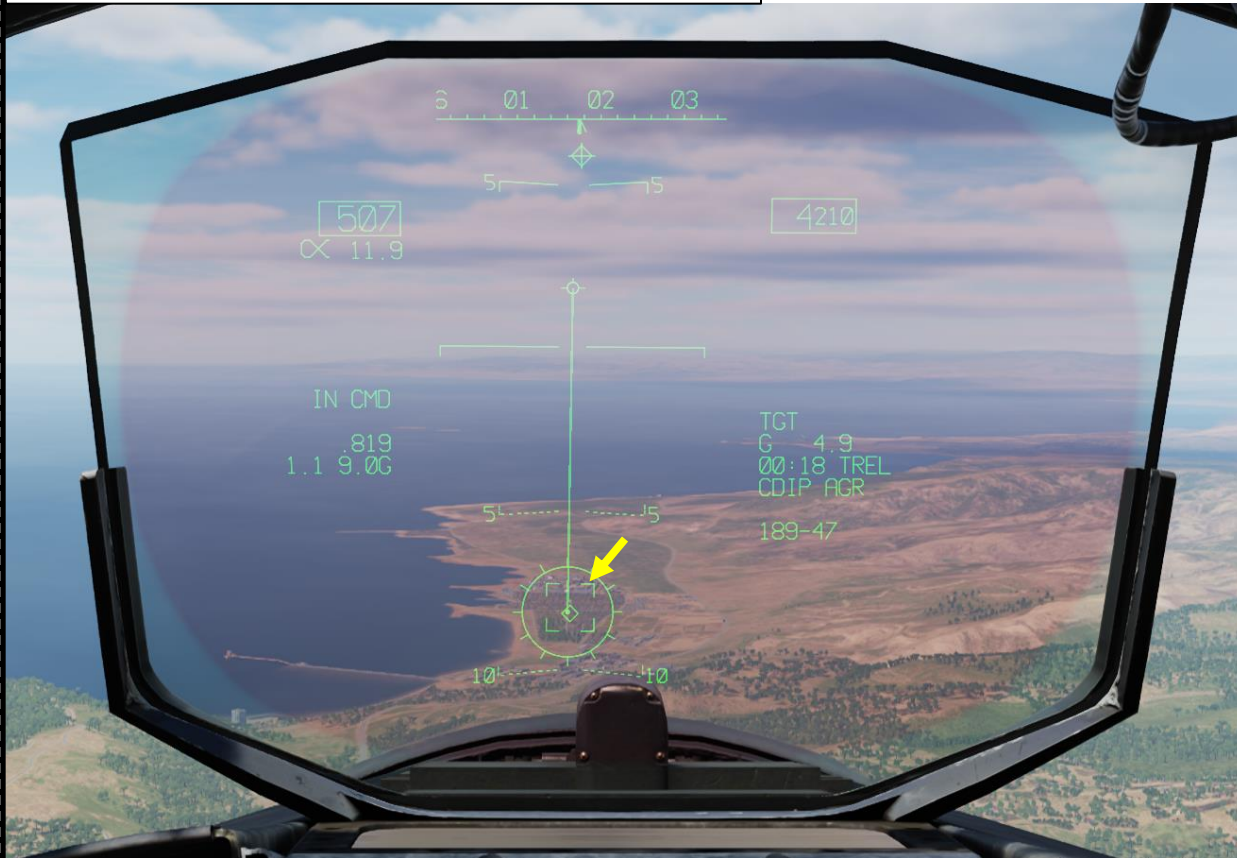
Targeting Pod Slaved to HUD Designation from CDIP (Continuously Displayed Impact Point) Mode Pipper/Reticle
