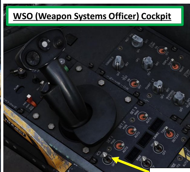
ICS (Internal Countermeasures Set) Mode Switch • FWD: Manual • MIDDLE: Automatic • AFT: Standby
