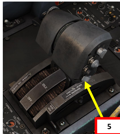
Weapon / Mode (Weapon Select) Switch • FWD: Medium Range Missile Selected • CENTER: Short Range Missile Selected • AFT: Auto Guns / A/A Mode Command Selected
