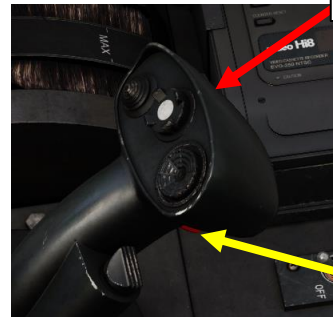
Left Hand Controller (LHC) Trigger • First Detent • Second Detent 1
