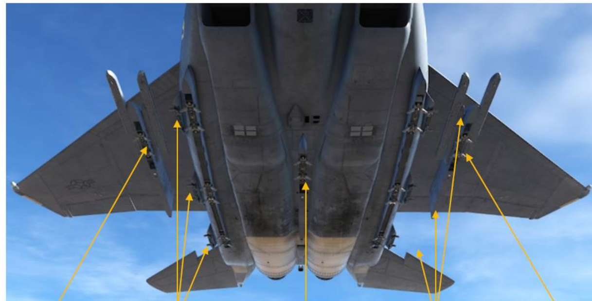
Station 8 Right CFT Station 5 Left CFT Station 2
